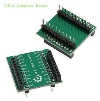
Introduction: This is a matching conversion board with hot sale product Xbee. It is very simple in design. This board converse all 20 pins of Xbee to double-row pins with 0.1 inches standard distance, the distance between the raws are 0.5 inches. Corresponding pins are marked out with corresponding screen printing, easy to identify. We use a female socket, so no need to solder XBee to the board. Features: 2 x10 20 pins.
